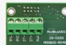
To connect Snow Depth Sensor to the motherboard, you will need **MOD BUS** interface.
